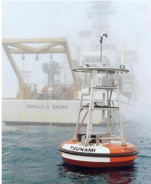
**Figure 14 - NOAA's DART buoy (picture for illustration)**
