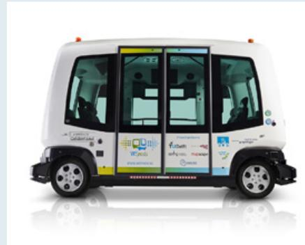
The WEpods come without driving wheel, brakes or accelerator pedals and are undergoing final tests on public roads in the provinces of Gelderland and the North Rhine-Westphalia, the Netherlands and Germany respectively – while similar driverless pods are already being used on dedicated lanes on Heathrow Airport and Rotterdam.
