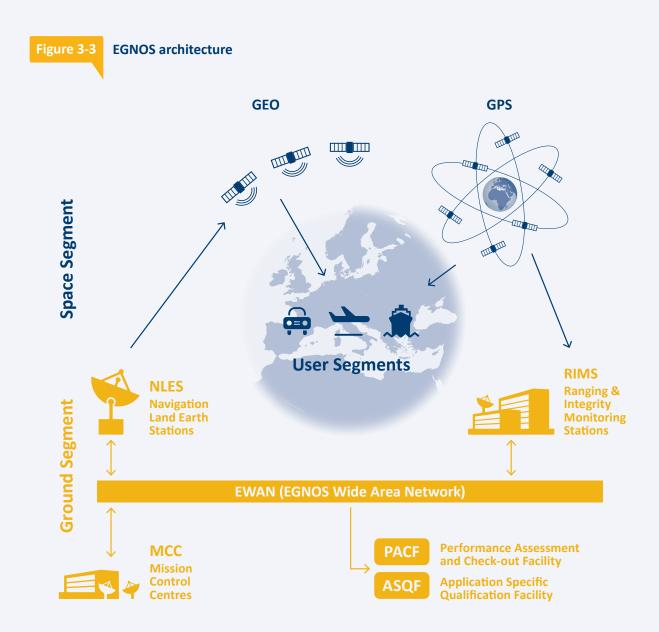
In order to provide its services to users equipped with appropriate receivers, the EGNOS system comprises two main segments: the Space Segment, and the Ground Segment.
