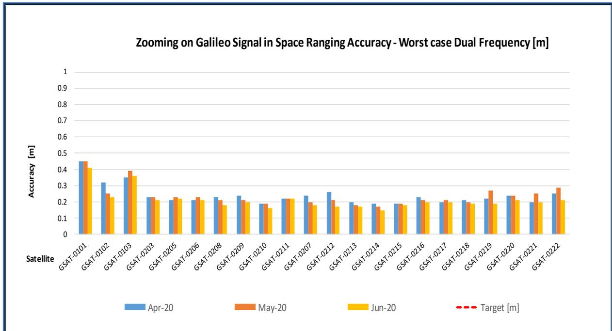
Figure 2 : Monthly Galileo SIS Ranging Accuracy (95<sup>th</sup> percentile) “for any satellite”, measured during reporting period for worst-case, Dual-Frequency (DF)
