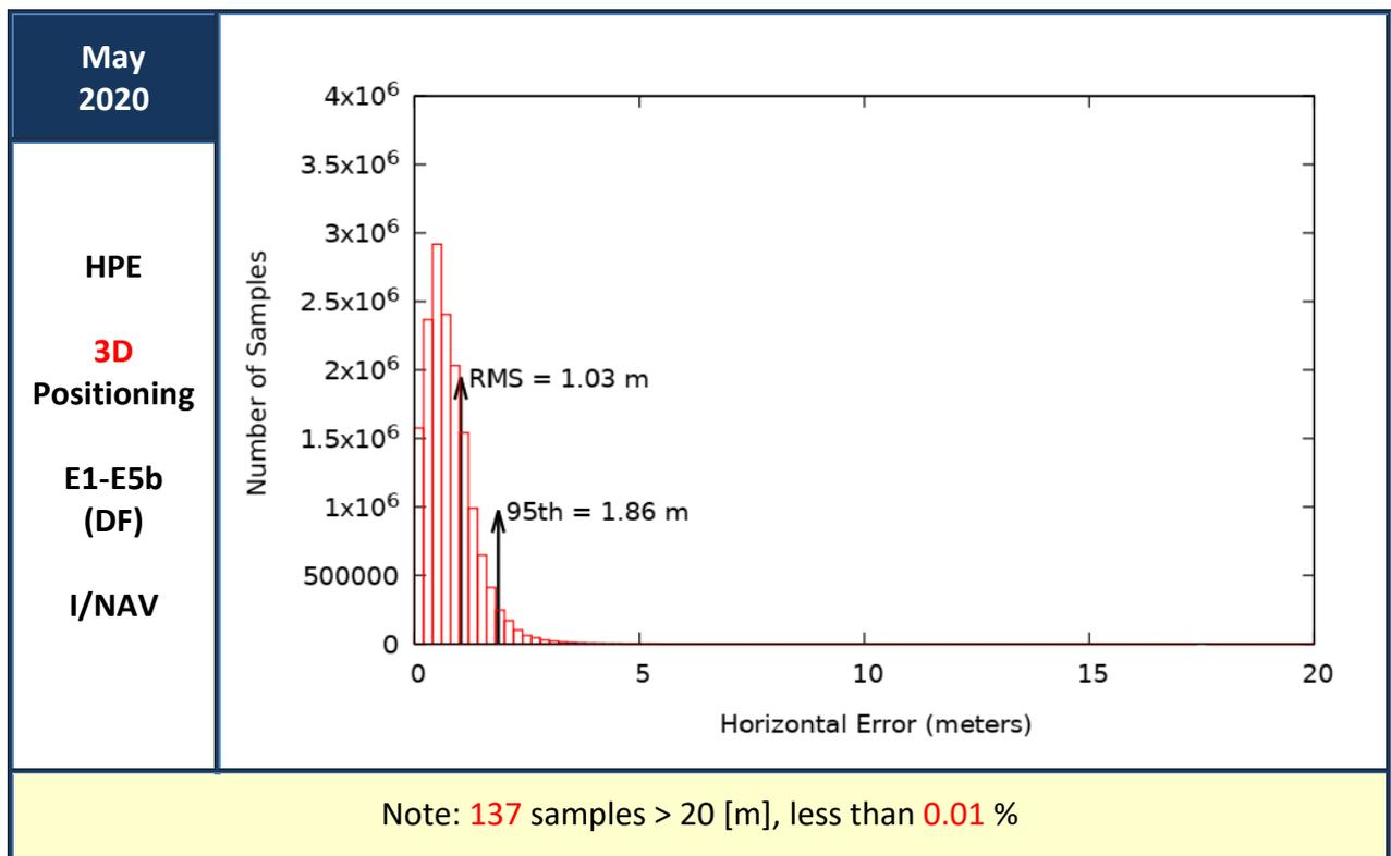
Figure 15 : Horizontal Positioning Error (HPE) for “Galileo-only” users in May 2020
