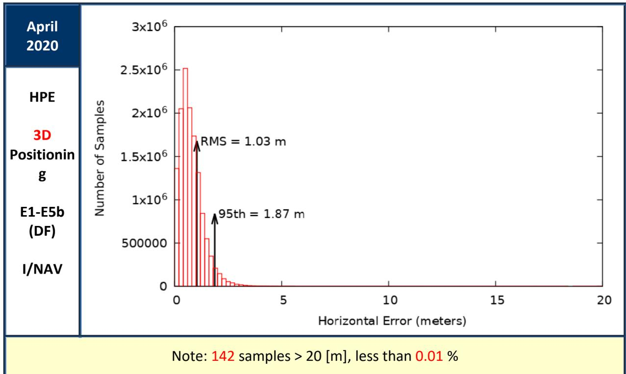
Figure 14 : Horizontal Positioning Error (HPE) for “Galileo-only” users in April 2020
