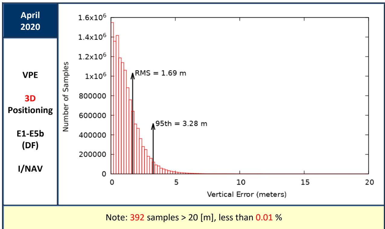
Figure 17 : Vertical Positioning Error (VPE) for “Galileo-only” users in April 2020
