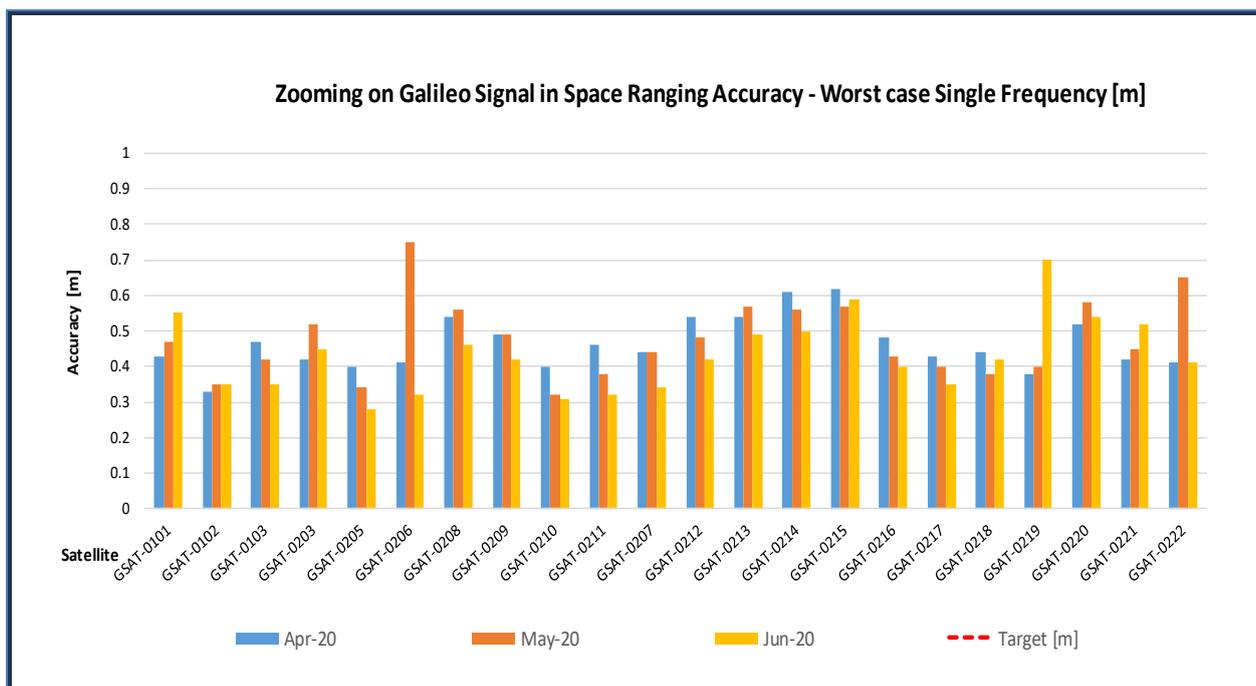
Figure 3 : Monthly Galileo SIS Ranging Accuracy (95<sup>th</sup> percentile) "for any satellite", measured during the reporting period for worst-case, Single-Frequency (SF)
