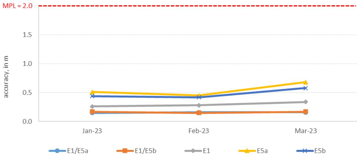
Figure 11: monthly Galileo signal in space ranging accuracy (95<sup>th</sup> percentile) over all satellites (constellation average), measured during the reporting period
