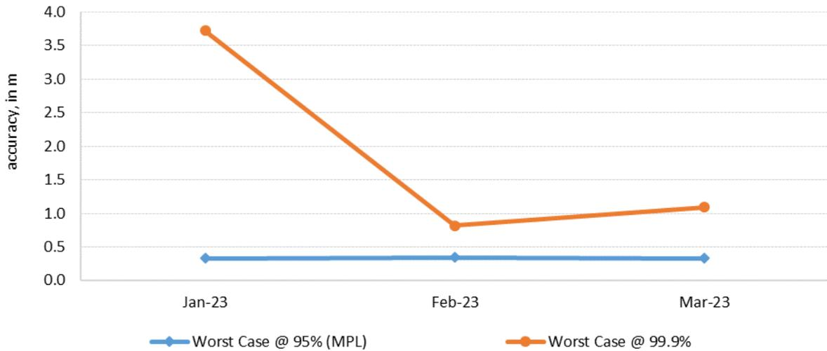
Figure 5: worst-case, monthly Galileo signal in space ranging accuracy (at 95<sup>th</sup> and 99.9<sup>th</sup> confidence level percentiles) for any satellite and any signal in space (dual frequency)
