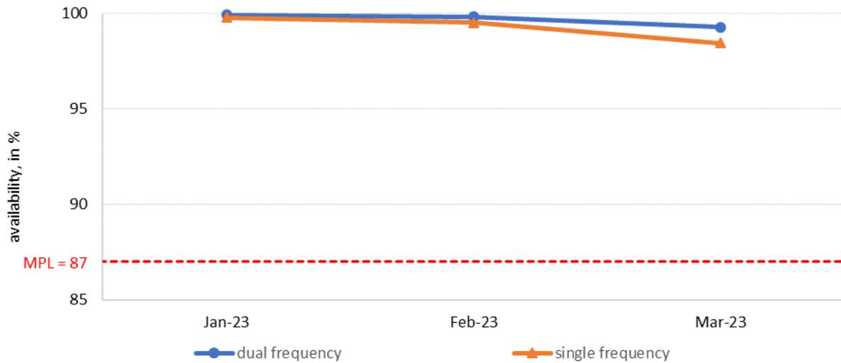
Figure 21: availability of positioning at Worst User Location (WUL) for single and dual frequency during the reporting period
