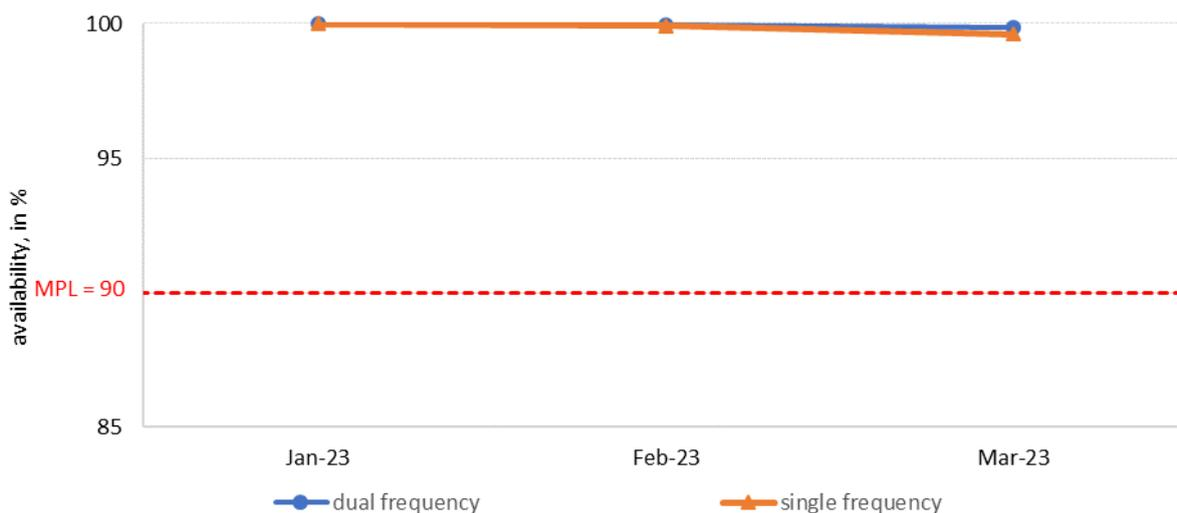
Figure 20: availability of positioning at Average User Location (AUL) for single and dual frequency during the reporting period
