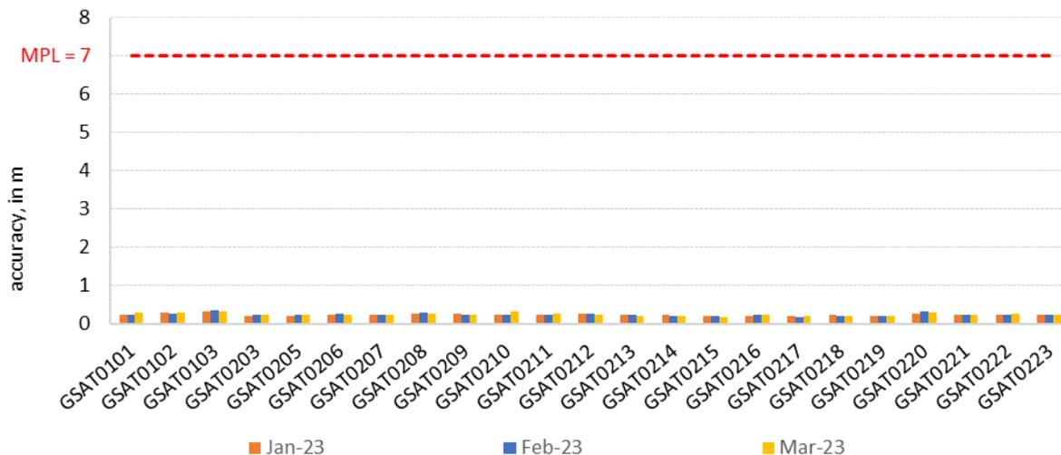
Figure 7: monthly Galileo signal in space ranging accuracy (95<sup>th</sup> percentile) for any satellite, measured during reporting period for worst-case (dual frequency) against MPL (minimum performance level)
