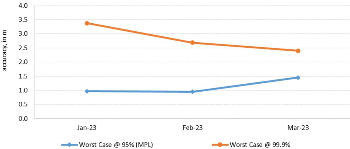
Figure 6: worst-case, monthly Galileo signal in space ranging accuracy (at 95<sup>th</sup> and 99.9<sup>th</sup> confidence level percentiles) for any satellite and any signal in space (single frequency)
