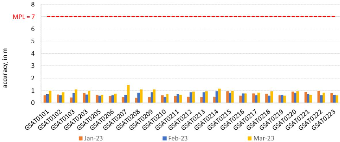
Figure 9: monthly Galileo signal in space ranging accuracy (95<sup>th</sup> percentile) for any satellite, measured during reporting period for worst-case (single frequency) against MPL (minimum performance level)
