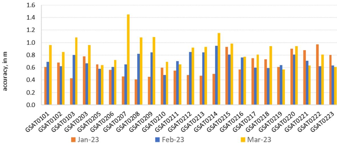
Figure 10: monthly Galileo signal in space ranging accuracy (95<sup>th</sup> percentile) for any satellite, measured during reporting period for worst-case (single frequency) – zoom in
