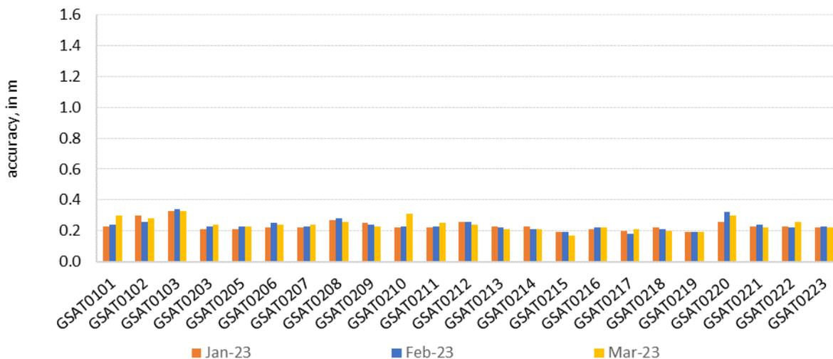
Figure 8: monthly Galileo signal in space ranging accuracy (95<sup>th</sup> percentile) for any satellite, measured during reporting period for worst-case (dual frequency) – zoom in
