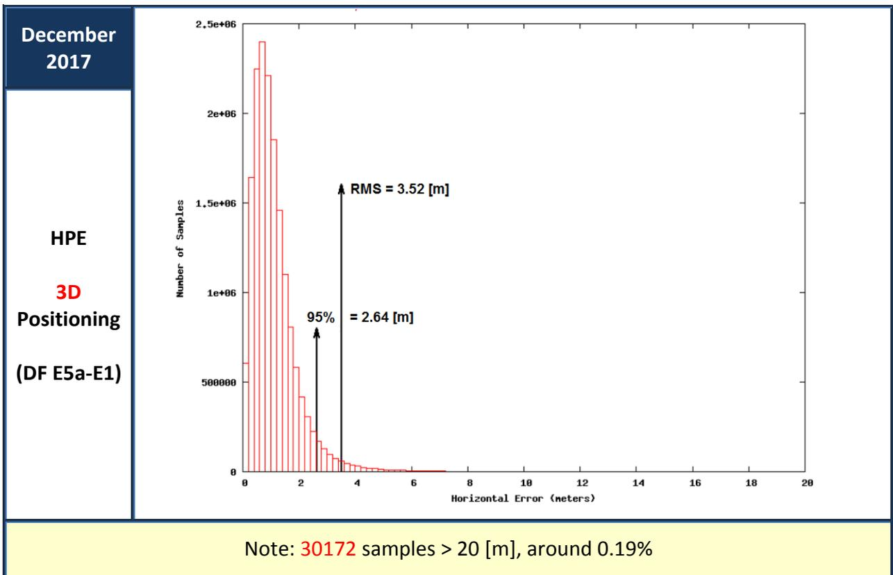
Figure 15: Horizontal Positioning Error (HPE) for “Galileo-only” users (December 2017)
