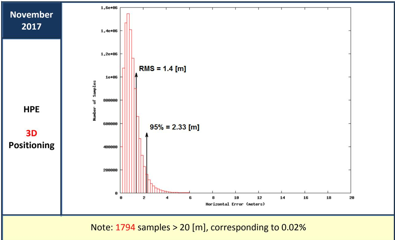
Figure 14: Horizontal Positioning Error (HPE) for “Galileo-only” users (November 2017)
