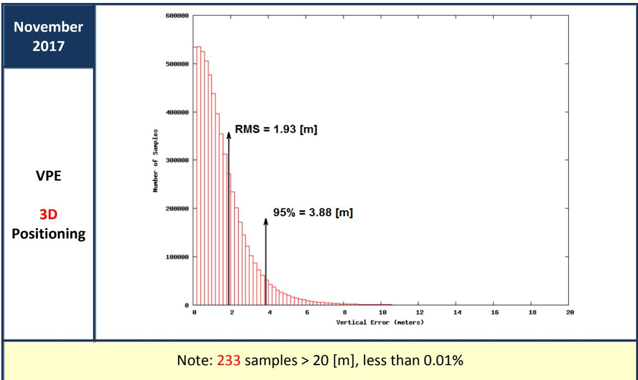
Figure 17: Vertical Positioning Error (VPE) for Galileo only users (November 2017)
