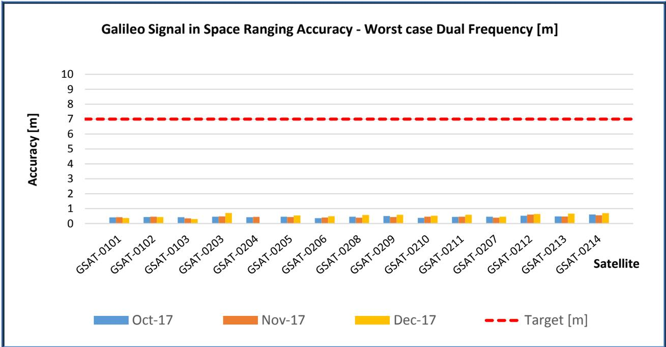
Figure 3: Monthly Galileo SIS Ranging Accuracy (95<sup>th</sup> percentile) “for any satellite”, measured during reporting period for worst-case, Dual-Frequency (DF)
