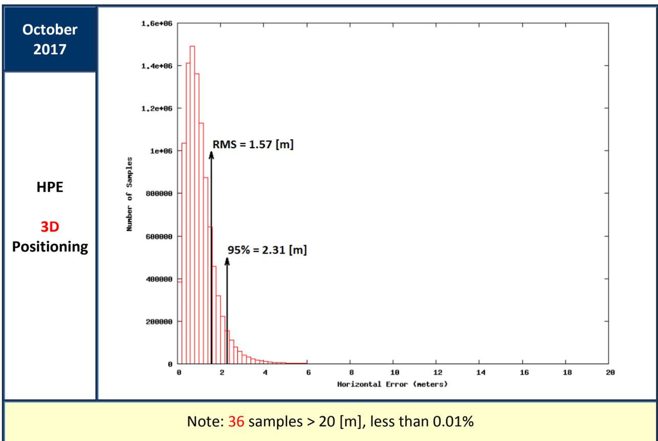
Figure 13: Horizontal Positioning Error (HPE) for "Galileo-only" users (October 2017)
