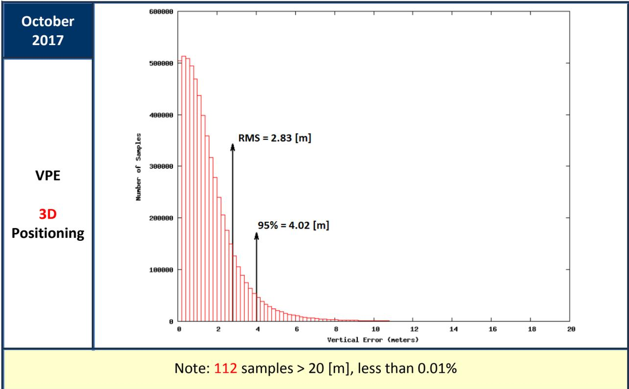
Figure 16: Vertical Positioning Error (VPE) for Galileo only users (October 2017)
