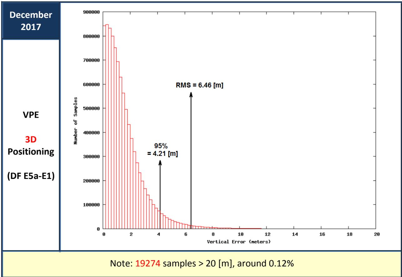
Figure 18: Vertical Positioning Error (VPE) for Galileo only users (December 2017)
