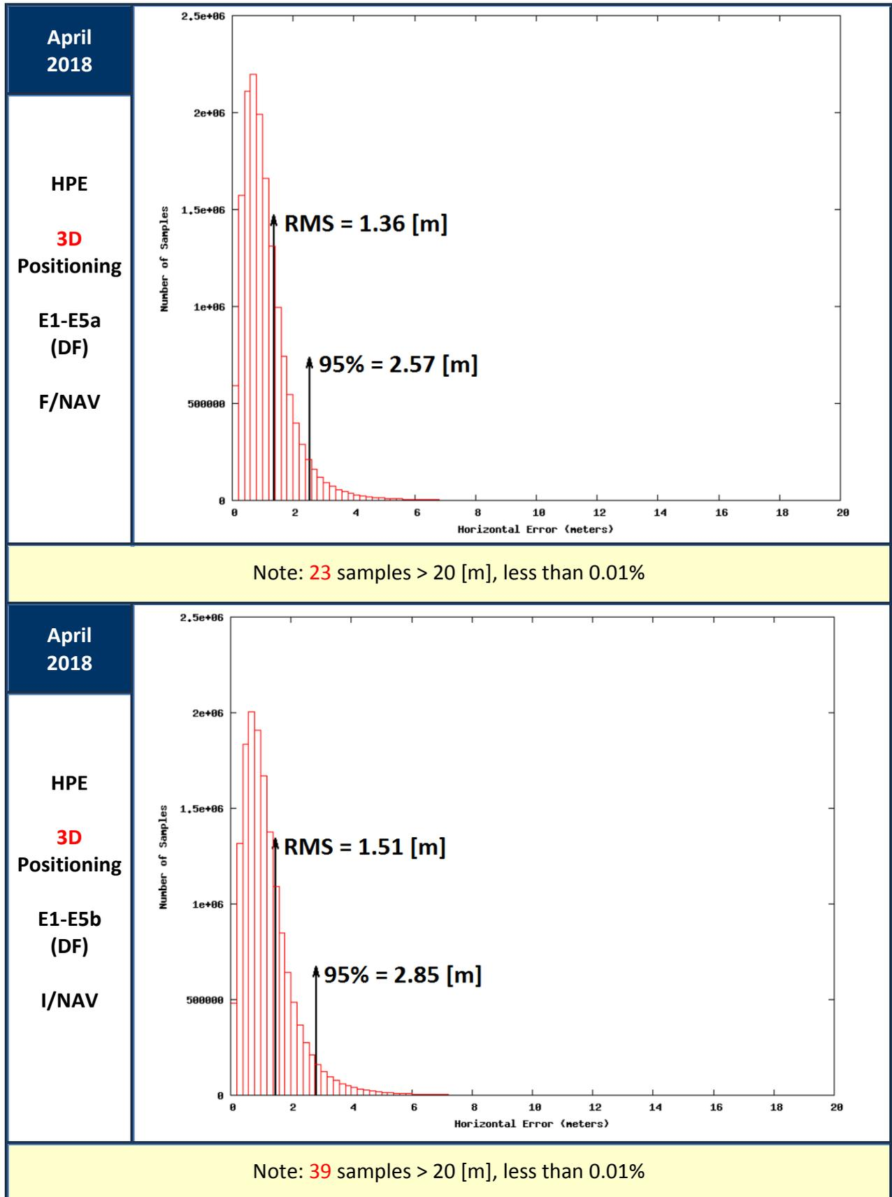
Figure 13: Horizontal Positioning Error (HPE) for “Galileo-only” users in April 2018
