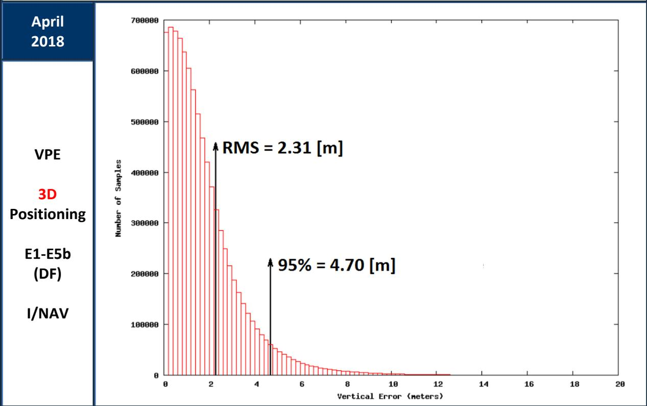
Figure 16: Vertical Positioning Error (VPE) for Galileo only users in April 2018
