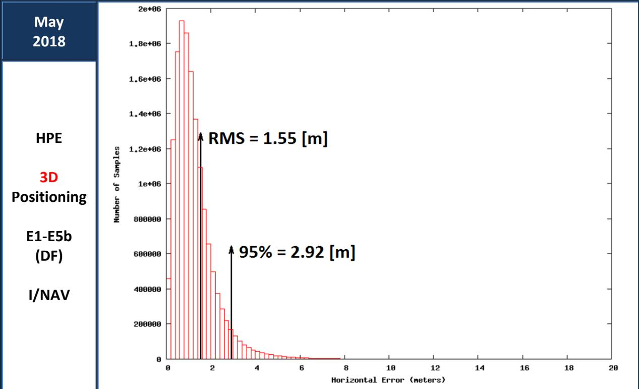
Figure 14: Horizontal Positioning Error (HPE) for “Galileo-only” users in May 2018
