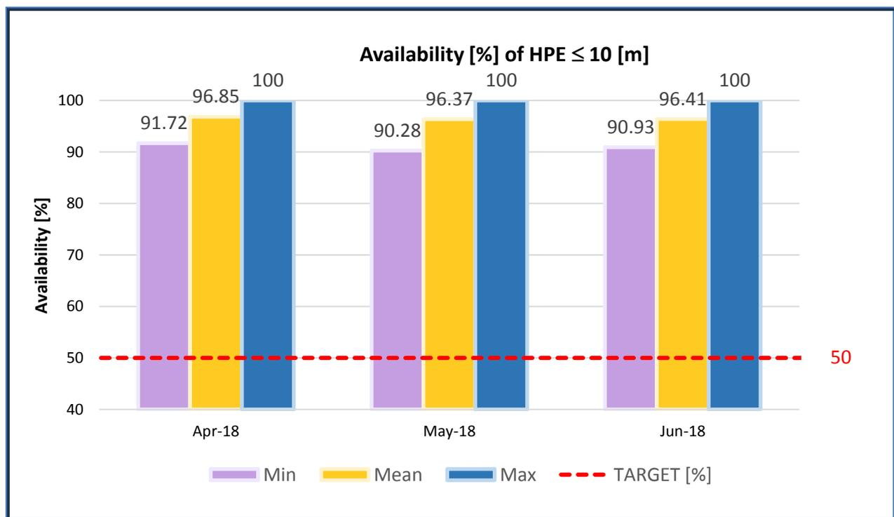
Figure 12: Availability of the Galileo Horizontal Positioning Service with Accuracy ≤ 10 [m]
