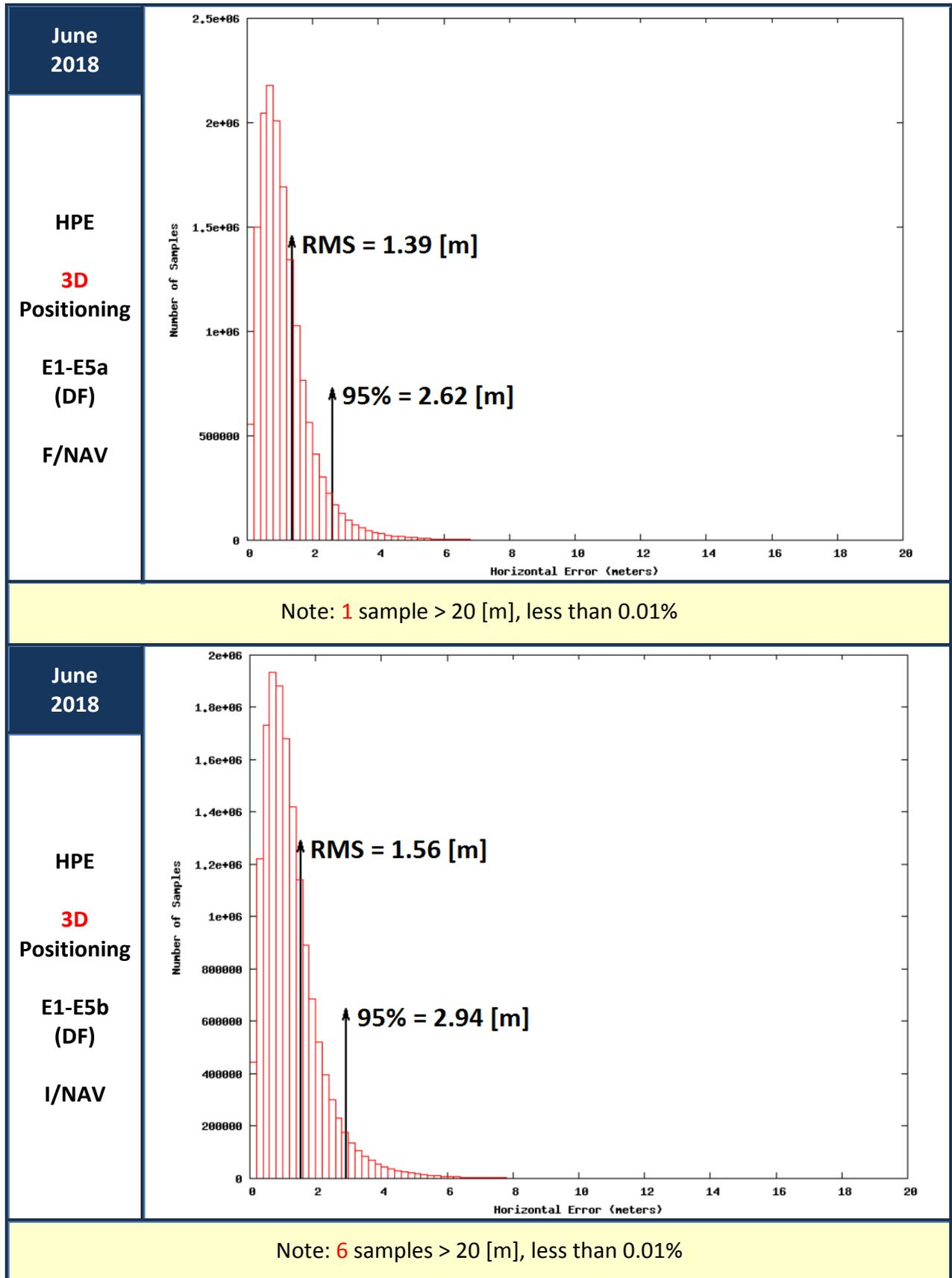
Figure 15: Horizontal Positioning Error (HPE) for “Galileo-only” users in June 2018
