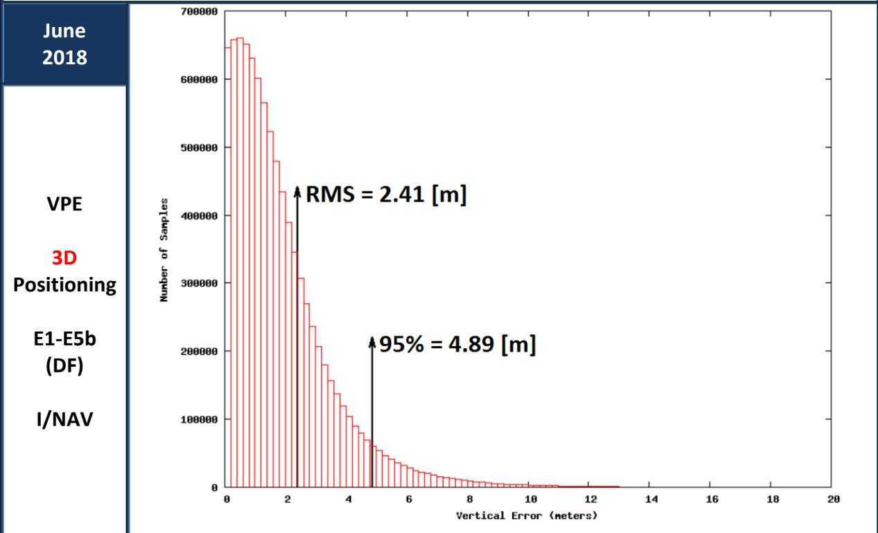
Figure 18: Vertical Positioning Error (VPE) for Galileo only users in June 2018
