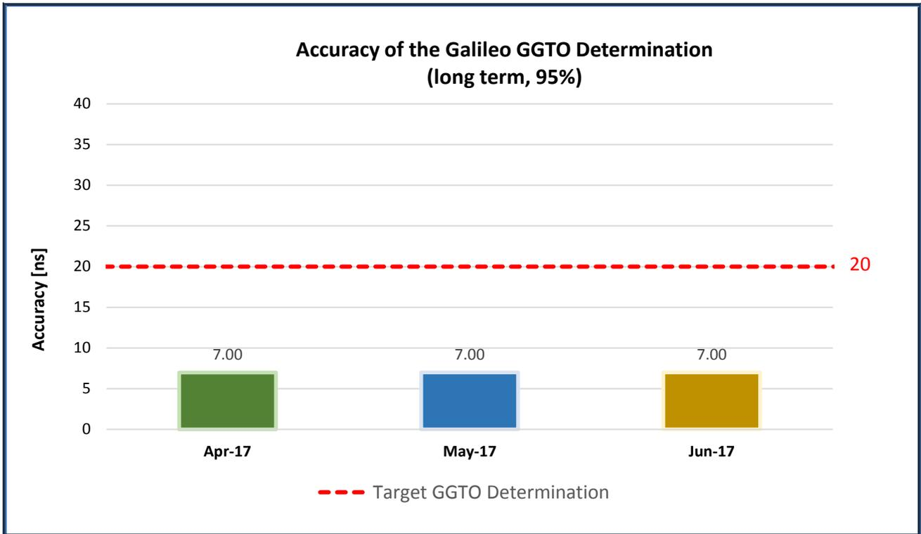
Figure 9: Long-term 95<sup>th</sup> percentile of GGTO Determination Accuracy
