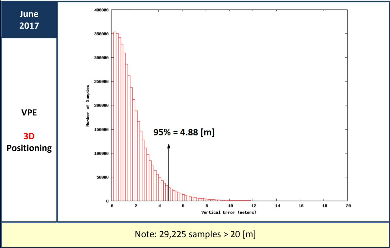
Figures 18: Vertical Positioning Error (VPE) for Galileo only users (June 2017)
