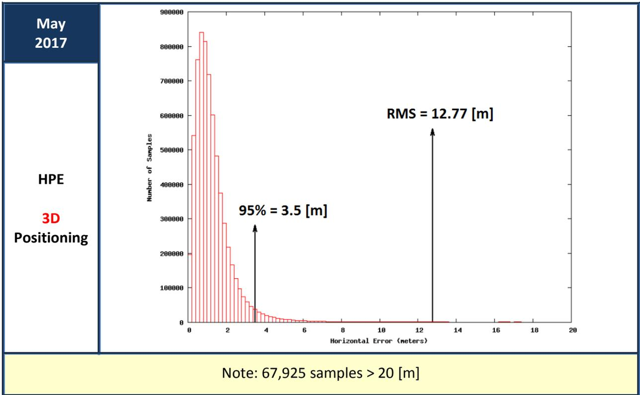
Figure 14: Horizontal Positioning Error (HPE) for “Galileo-only” users (May 2017)
