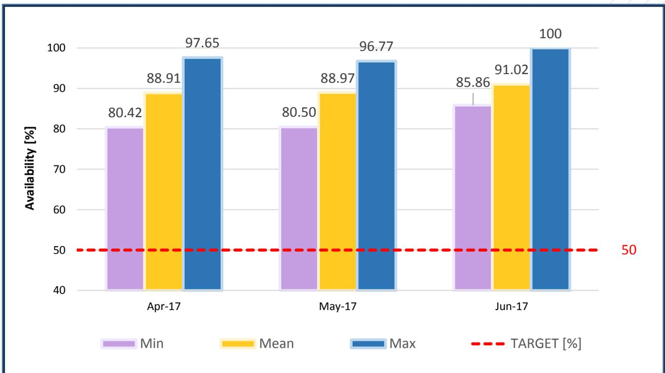
Figure 12: Availability of the Galileo Horizontal Positioning Service with Accuracy  $\leq 10$  [m]
