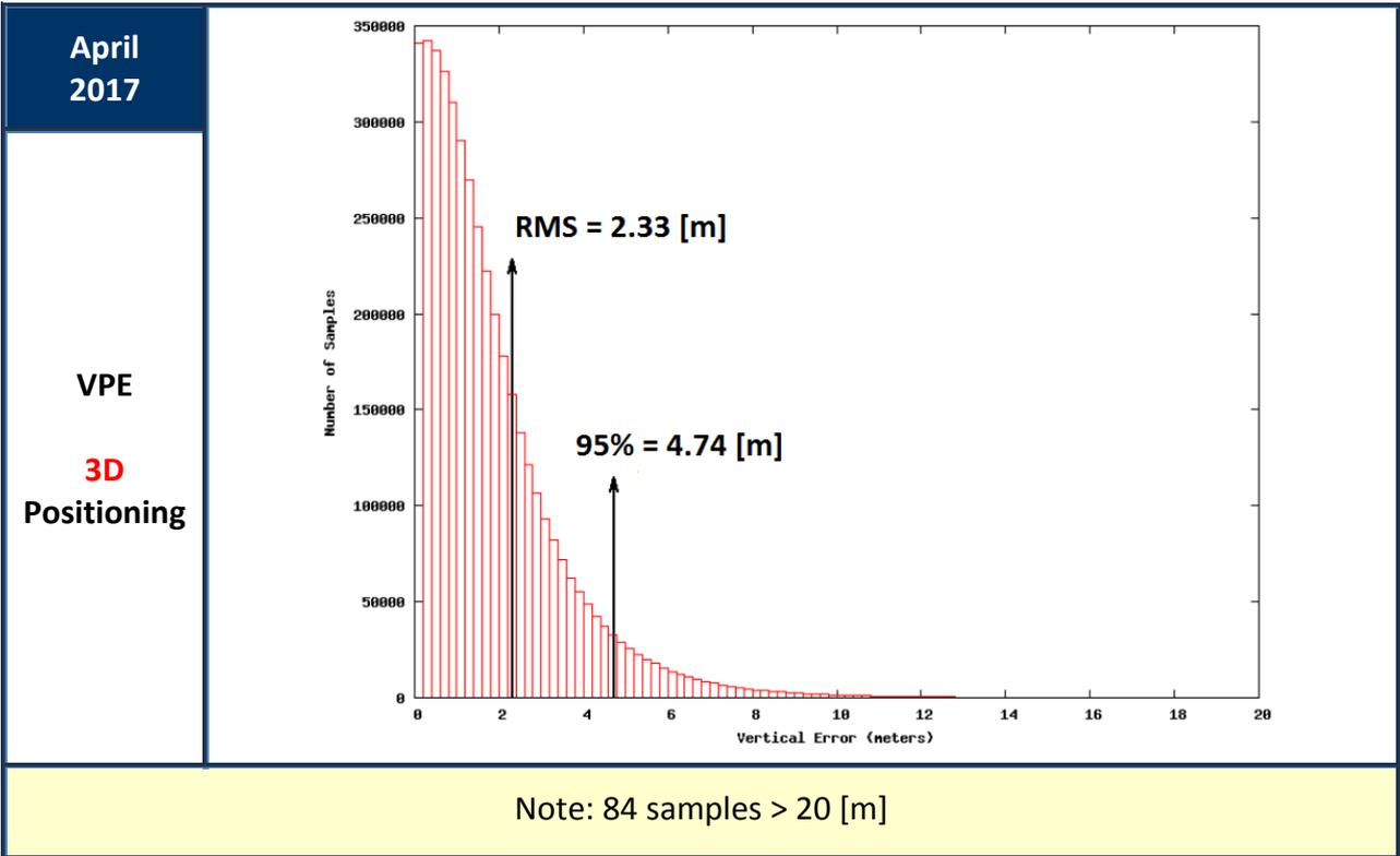
Figures 16: Vertical Positioning Error (VPE) for Galileo only users (April 2017)
