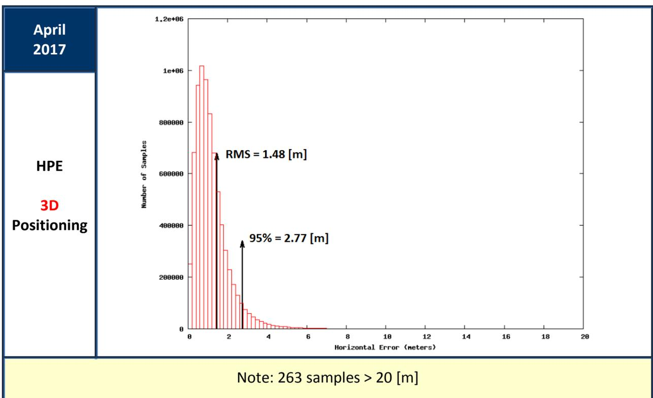
Figure 13: Horizontal Positioning Error (HPE) for "Galileo-only" users (April 2017)
