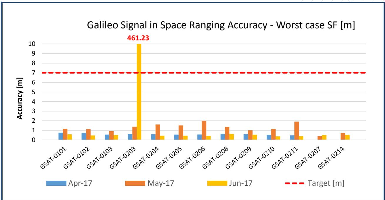
Figure 4: Monthly Galileo SIS Ranging Accuracy (95<sup>th</sup> percentile) “for any satellite”, measured during reporting period for worst-case, Single-Frequency (SF)
