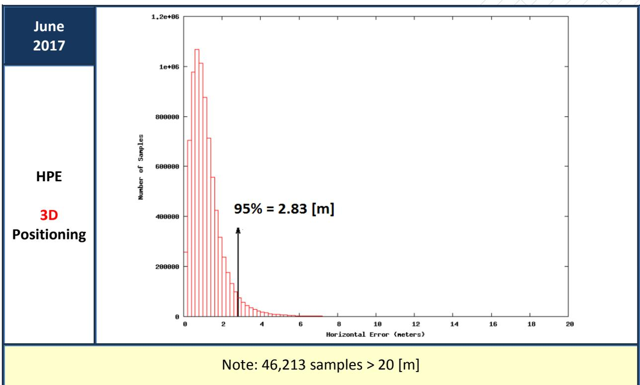
Figure 15: Horizontal Positioning Error (HPE) for “Galileo-only” users (June 2017)
