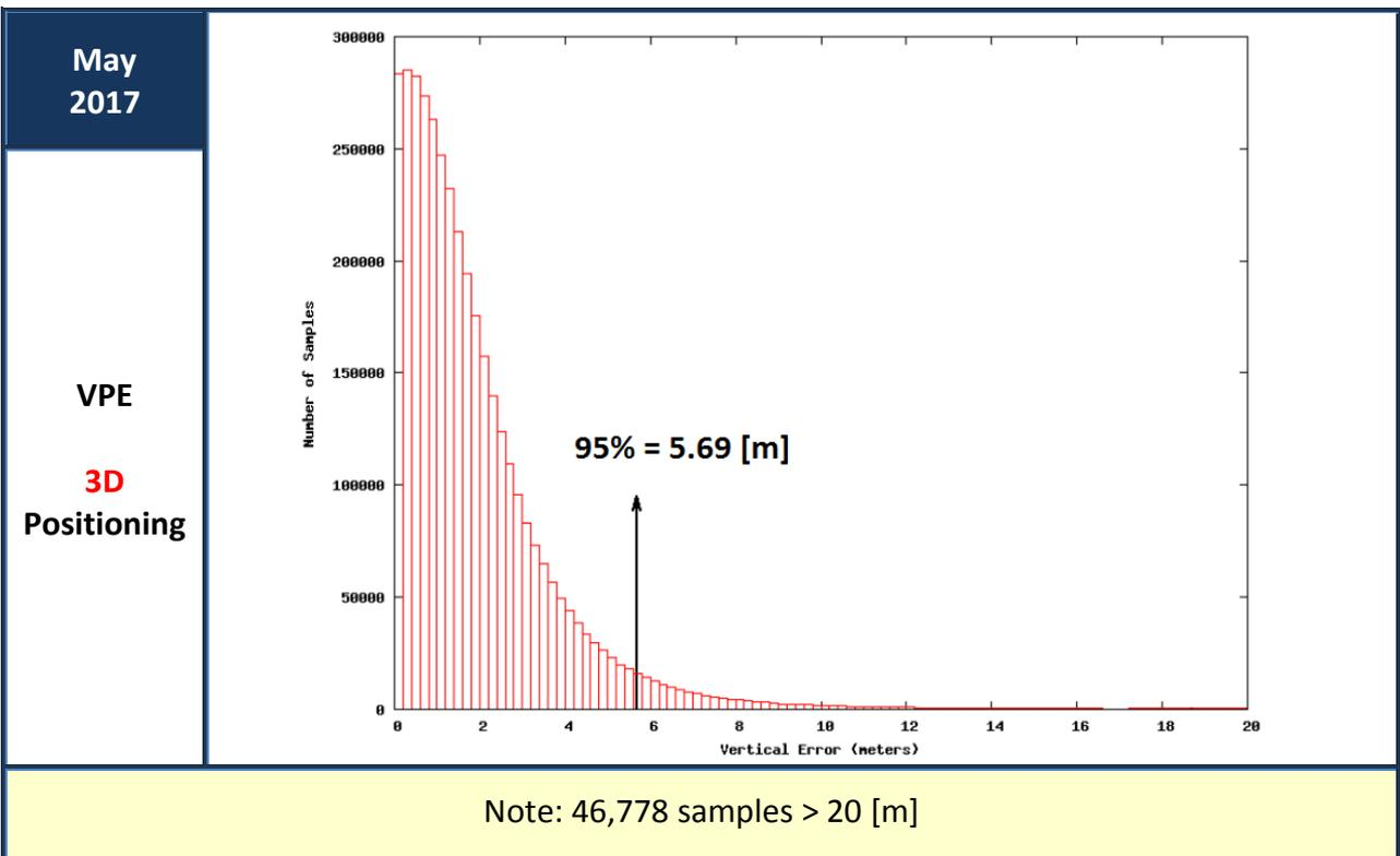
Figures 17: Vertical Positioning Error (VPE) for Galileo only users (May 2017)
