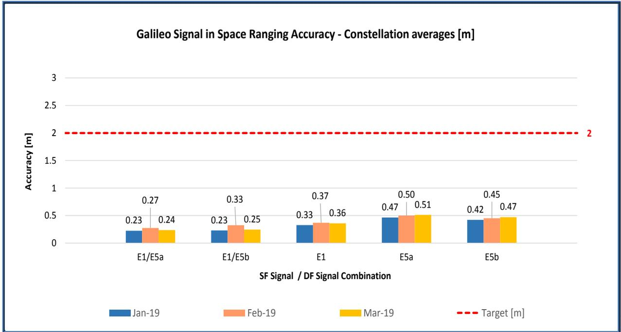
Figure 5: Monthly Galileo SIS Ranging Accuracy (95<sup>th</sup> percentile) “over all satellites” (constellation average), measured during the reporting period
