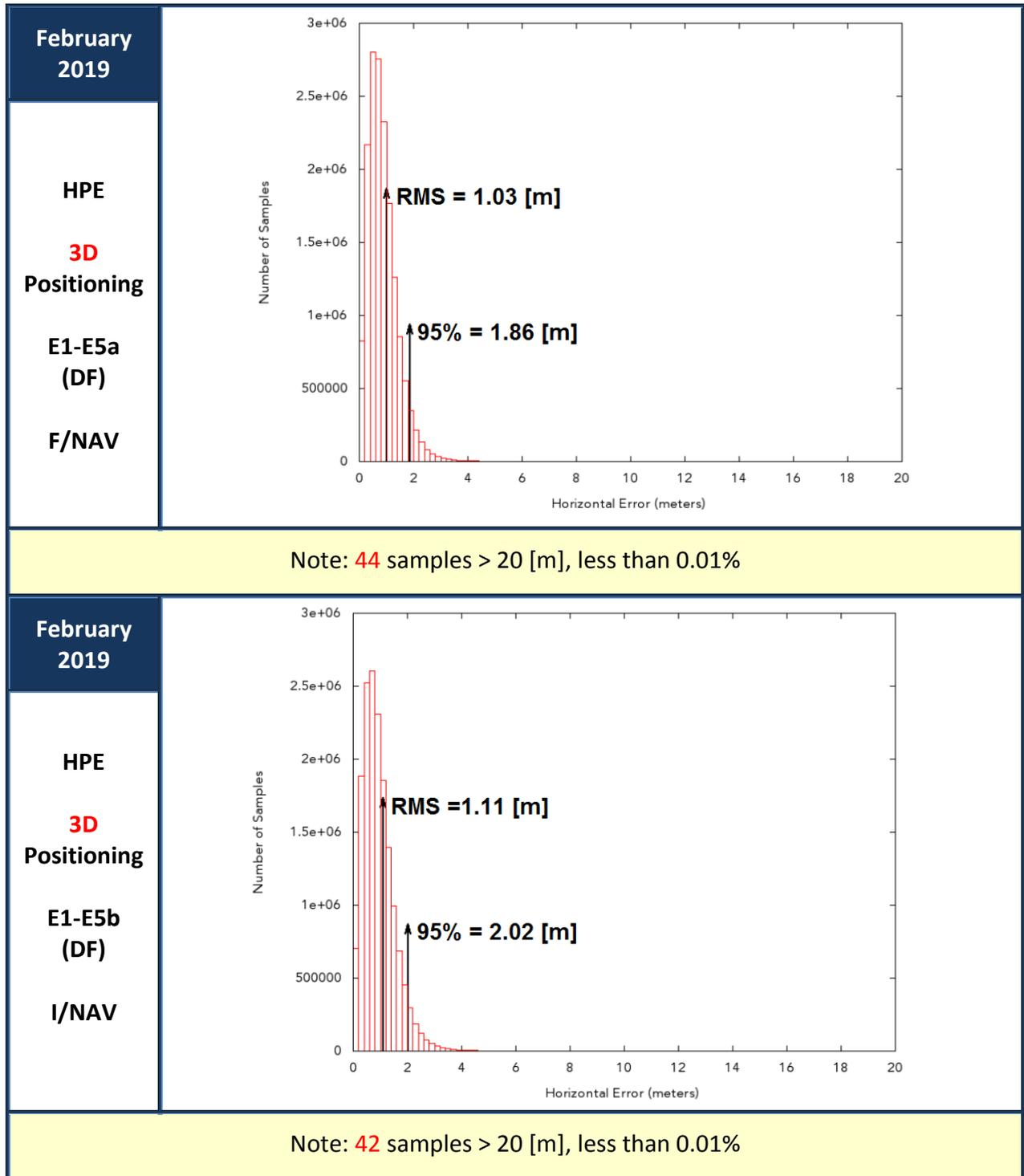
Figure 14: Horizontal Positioning Error (HPE) for “Galileo-only” users in February 2019
