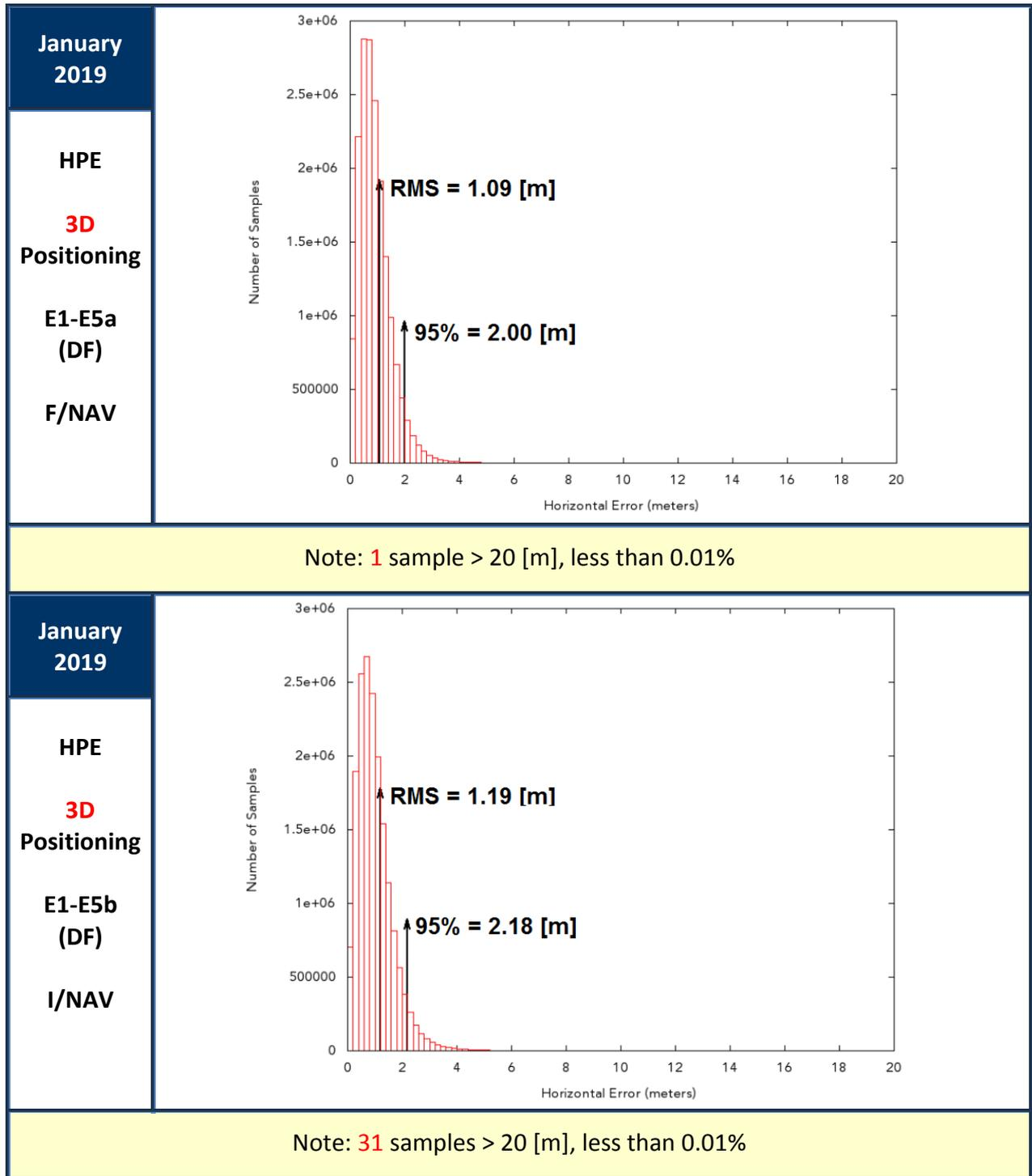
Figure 13: Horizontal Positioning Error (HPE) for “Galileo-only” users in January 2019
