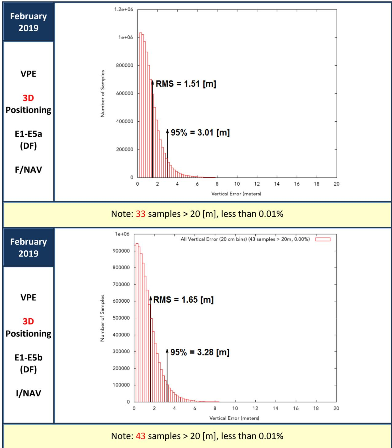
Figure 17: Vertical Positioning Error (VPE) for “Galileo-only” users in February 2019
