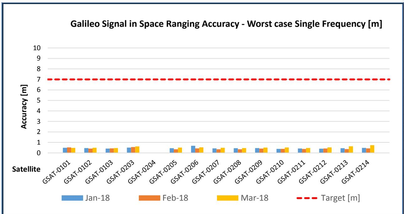
Figure 4: Monthly Galileo SIS Ranging Accuracy (95<sup>th</sup> percentile) "for any satellite", measured during the reporting period for worst-case, Single-Frequency (SF)
