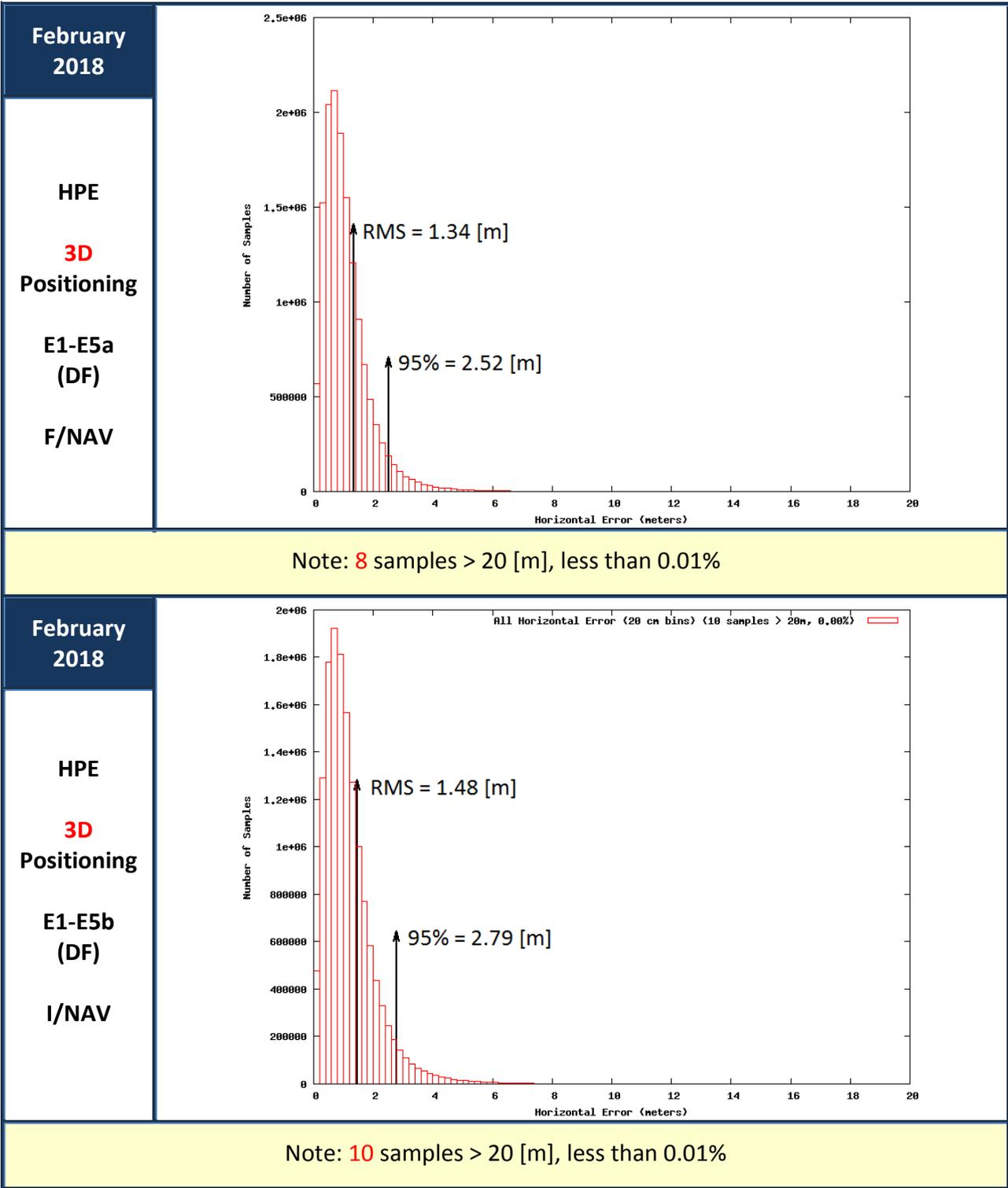
Figure 14: Horizontal Positioning Error (HPE) for “Galileo-only” users in February 2018
