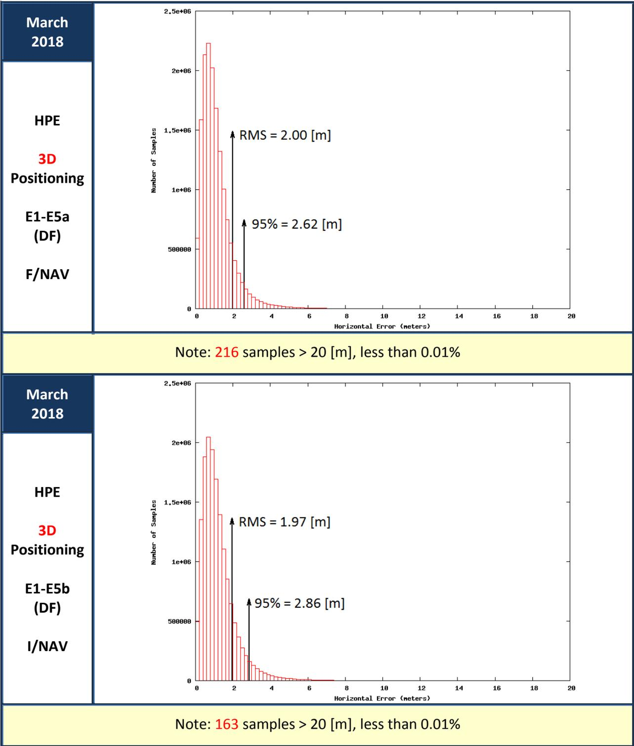
Figure 15: Horizontal Positioning Error (HPE) for “Galileo-only” users in March 2018
