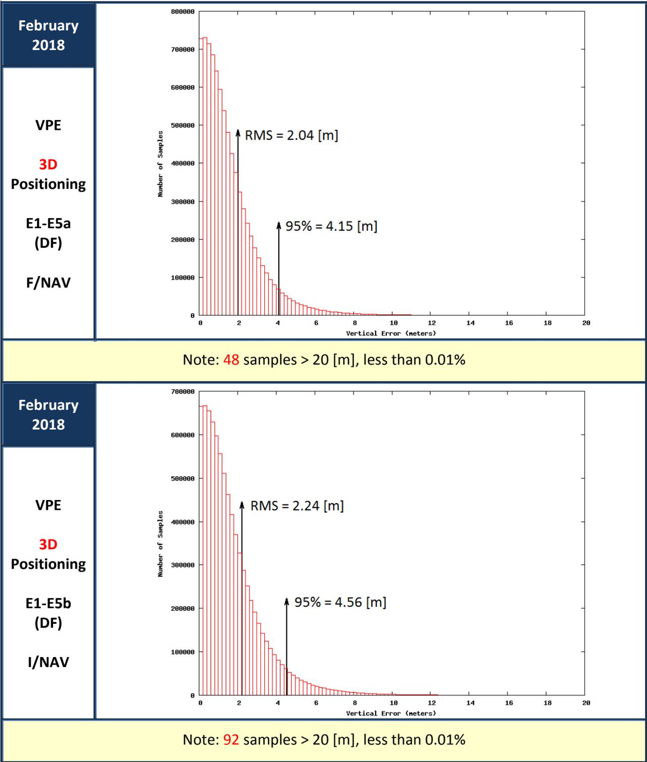
Figure 17: Vertical Positioning Error (VPE) for Galileo only users in February 2018
