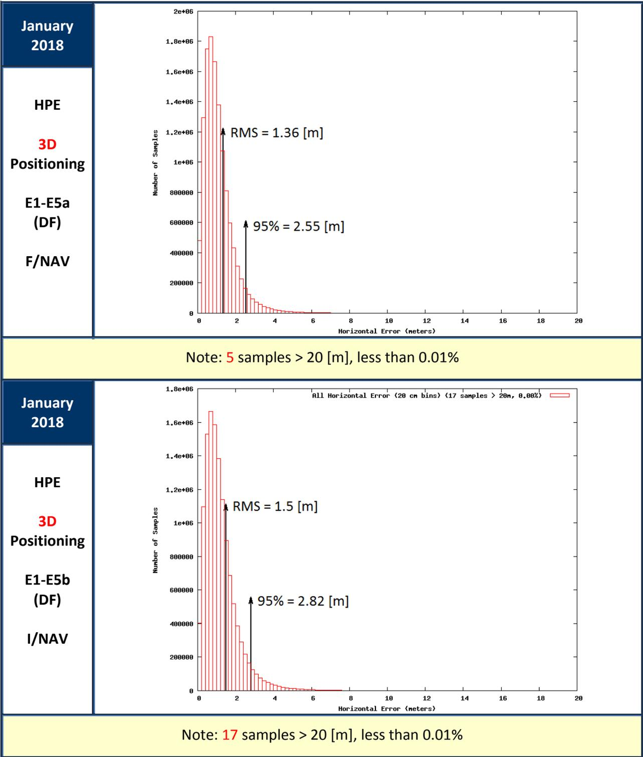
Figure 13: Horizontal Positioning Error (HPE) for “Galileo-only” users in January 2018
