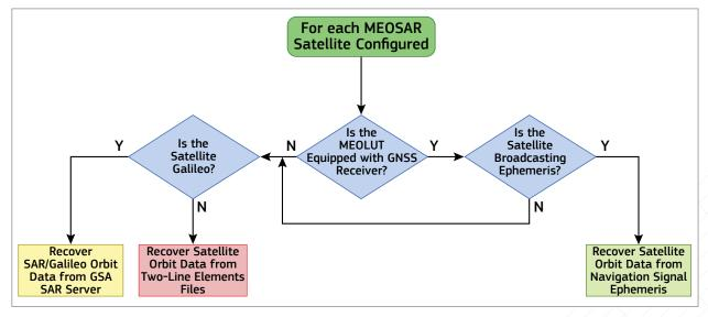
Figure 19. EU/MEOLUT satellite orbit data recovery process.
