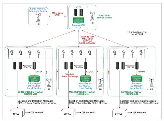
Figure 9. SAR/Galileo Ground Segment Overall Architecture.
