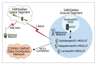
Figure 6. SAR/Galileo architecture.
