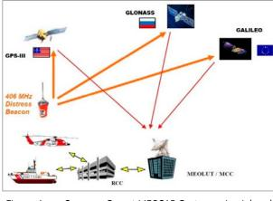
Figure 4. Cospas – Sarsat MEOSAR System using L band satellites.
