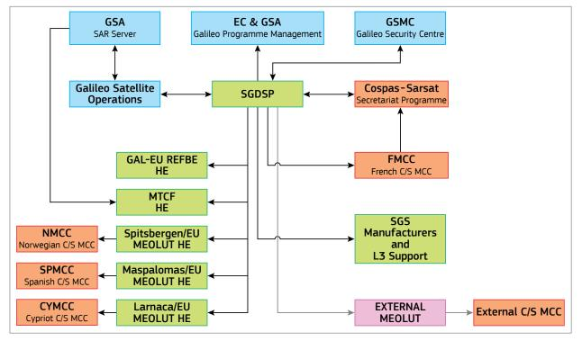
Figure 15. Interfaces of the SAR/Galileo Operations.
