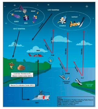
Figure 3. Description of LEOSAR and GEOSAR system.
