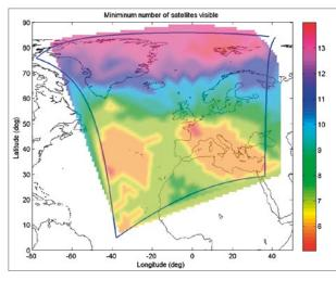
Figure 26. Minimum number of visible satellites for full SAR/Galileo constellation.
