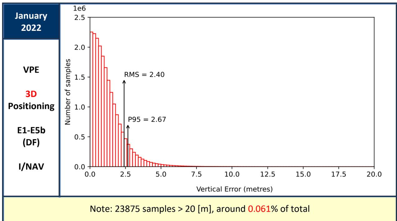
Figure 22 : Vertical Positioning Error (VPE) for “Galileo-only” users in January 2022
