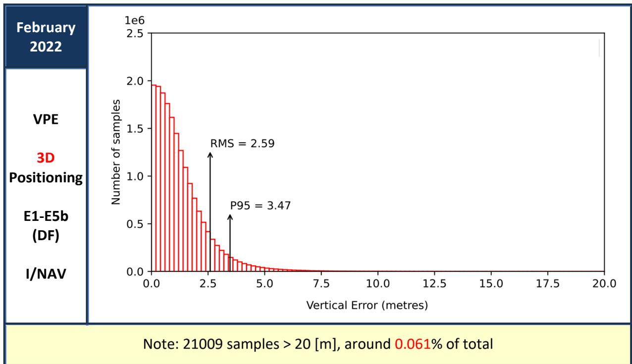
Figure 23 : Vertical Positioning Error (VPE) for “Galileo-only” users in February 2022
