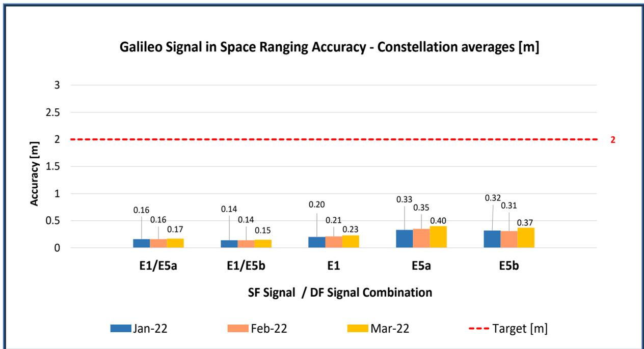
Figure 8 : Monthly Galileo SIS Ranging Accuracy (95<sup>th</sup> percentile) “over all satellites” (constellation average), measured during the reporting period
