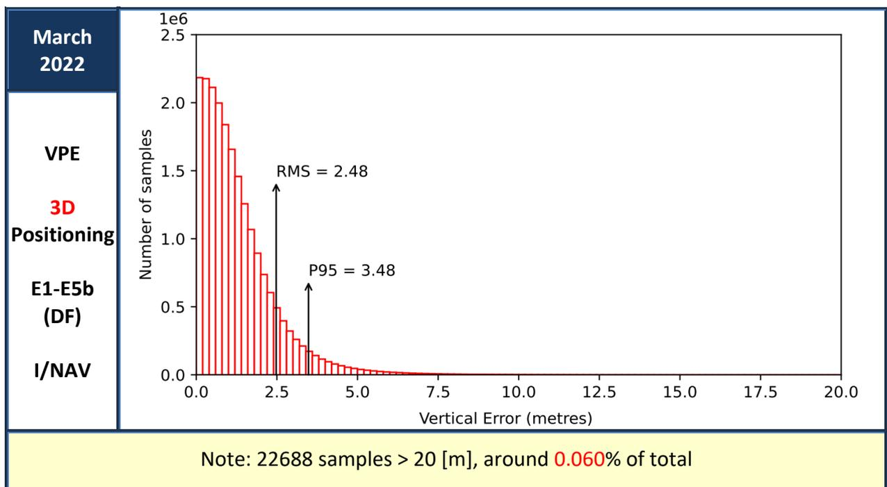
Figure 24 : Vertical Positioning Error (VPE) for “Galileo-only” users in March 2022
