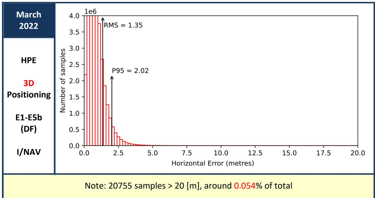
Figure 21 : Horizontal Positioning Error (HPE) for “Galileo-only” users in March 2022
