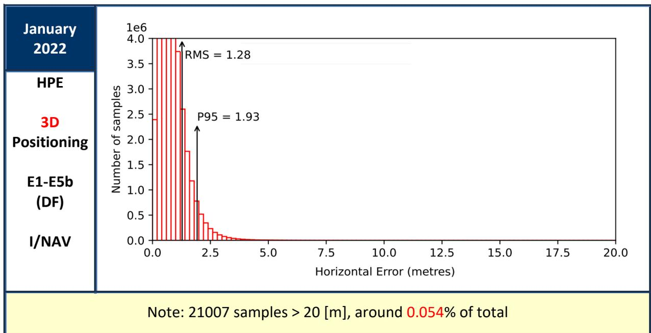
Figure 19 : Horizontal Positioning Error (HPE) for “Galileo-only” users in January 2022
