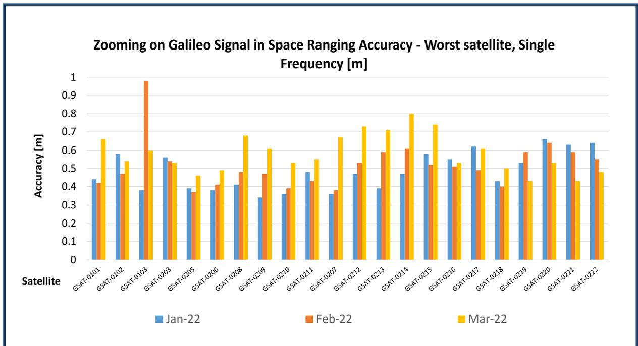
Figure 7 : Monthly Galileo SIS Ranging Accuracy (95<sup>th</sup> percentile) "for any satellite", measured during the reporting period for worst-case, Single-Frequency (SF)
