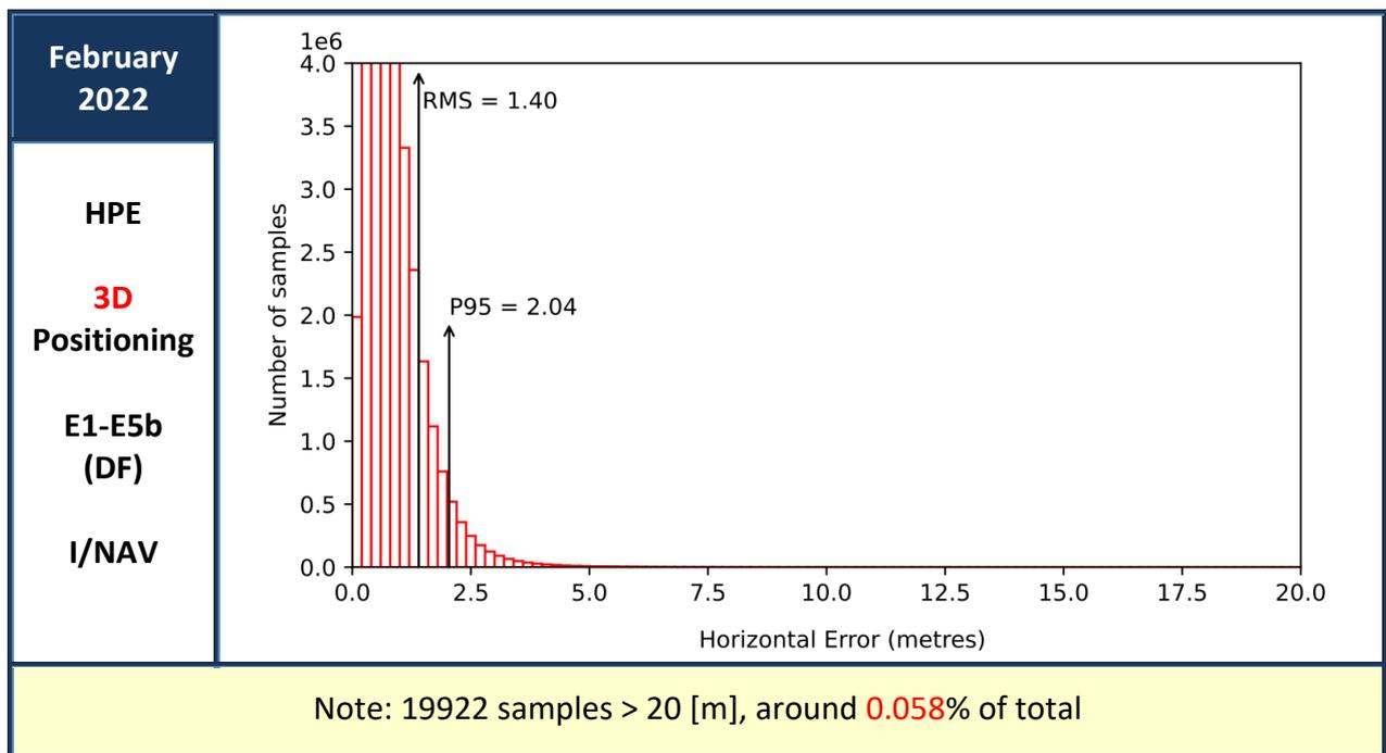
Figure 20 : Horizontal Positioning Error (HPE) for “Galileo-only” users in February 2022
