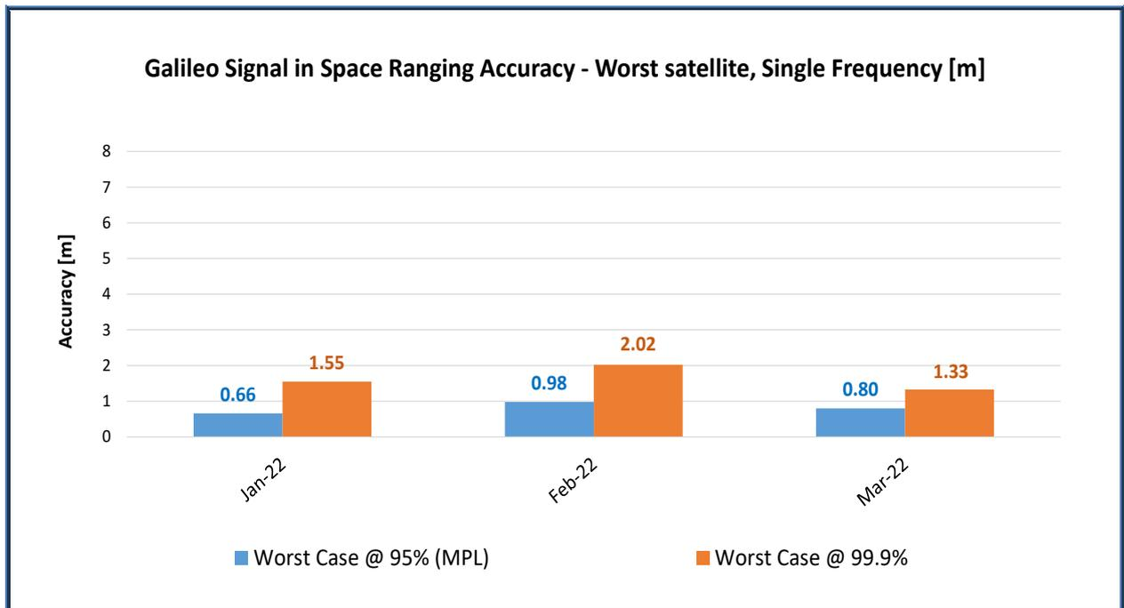
Figure 5 : Worst-case, monthly Galileo SIS Ranging Accuracy (at 95<sup>th</sup> and 99.9<sup>th</sup> confidence level percentiles) “for any satellite”, any SIS (SF and DF combinations)
