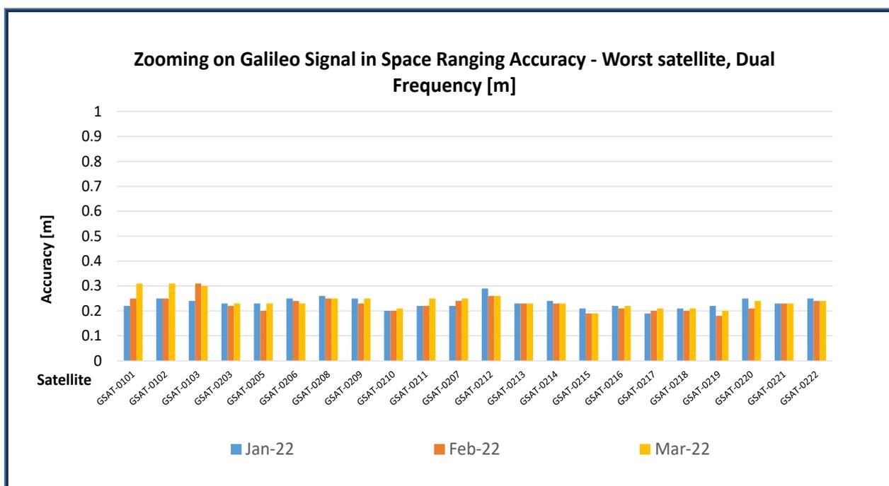
Figure 6 : Monthly Galileo SIS Ranging Accuracy (95<sup>th</sup> percentile) “for any satellite”, measured during reporting period for worst-case, Dual-Frequency (DF)
