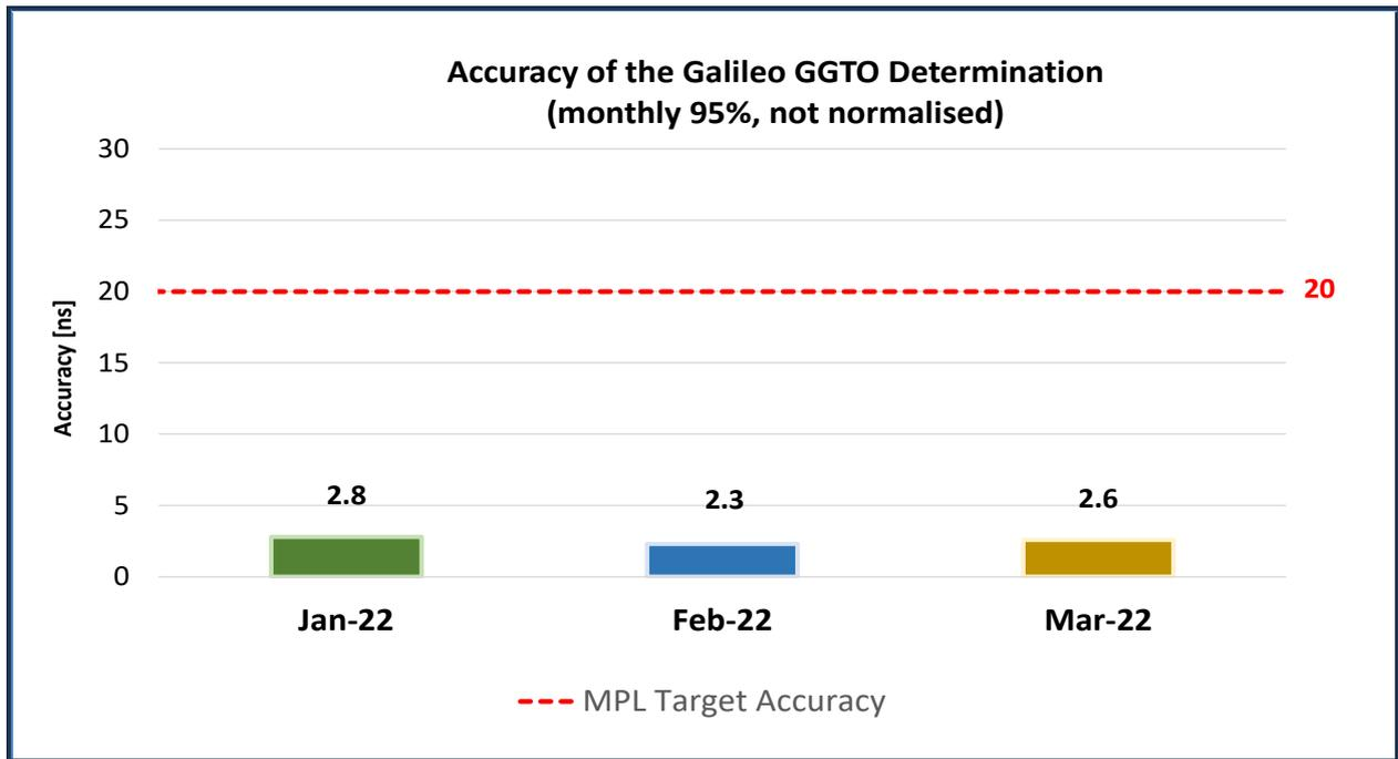
Figure 14 : Long-term 95<sup>th</sup> percentile of GGTO Determination Accuracy
