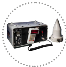
TI-4100 NAVSTAR GPS Receiver, 1981 One of the first commercial GPS receivers.
